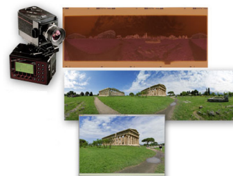
Figure 1. Seitz 220VR rotational film camera. Top to bottom, example of a negative, spanning 410 degrees, from Seitz camera (using 20mm lens). Positive after scanning, and cropping to 360 degrees. The cylindrical perspective results from the use of a rotational camera.
